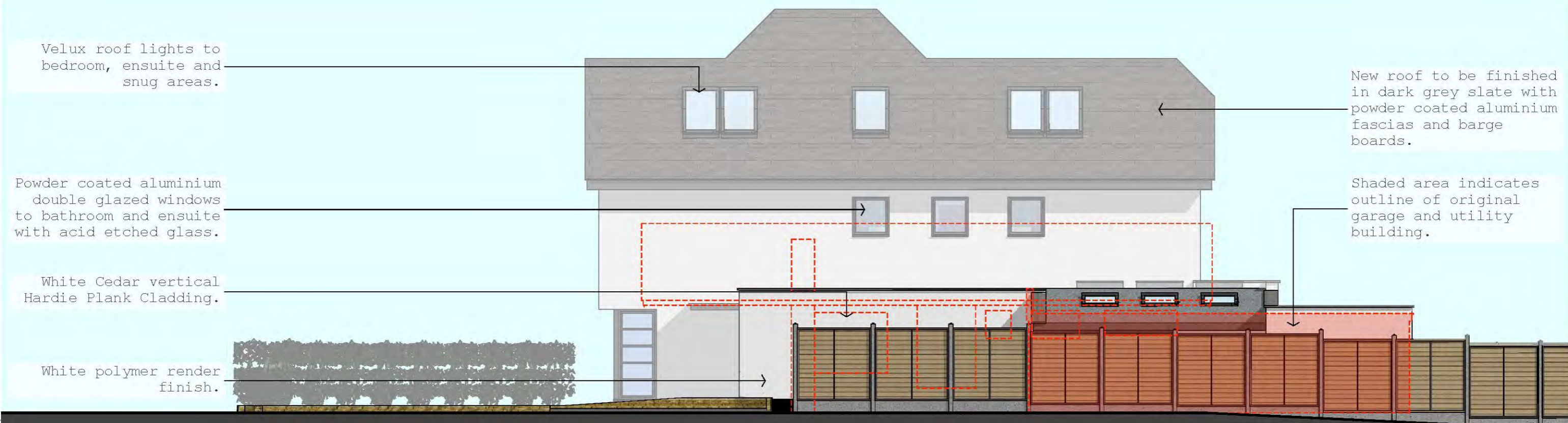
Side (north) Elevation as proposed
